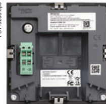
Connection with FDM121 display unit
