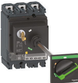
ComPacT NSX with an extended rotary handle installed at the back of a switchboard, with the keylock option and key
